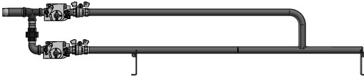
Figure 8-5 _Gas Train 500,000 Btu/hr Model
